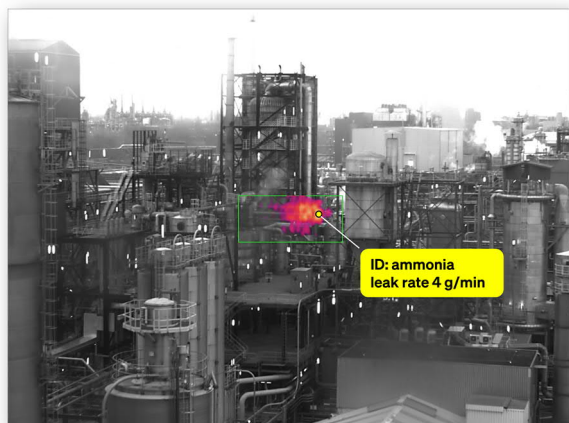
Figure 4: Detection of small leaks in a production facility at 200 m distance.
