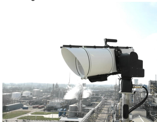
Figure 2: The scanfeld® sensor unit in a chemical park. In this installation two sensors monitor four production facilities. The sensor units have flexible scan ranges in 360°. The monitoring solution works autonomously 24/7.
