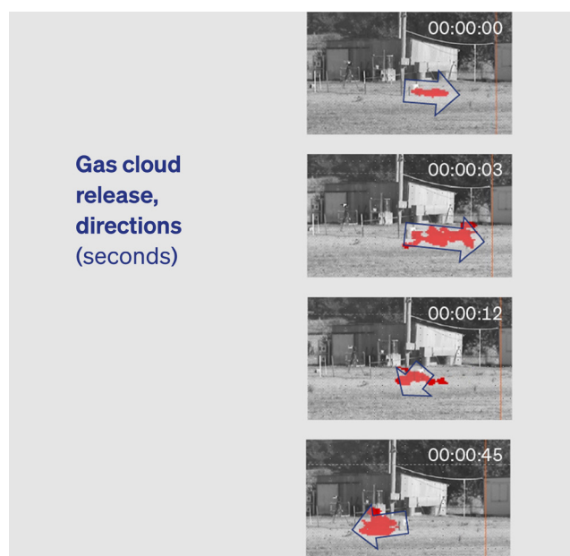
Figure 2. Field experiment with methane release: it is practically impossible to place a gas sensor in the best position. (Distribution of a cloud caused by a small leak [20 g/min.], measured with a Bruker spectrometer). 2
