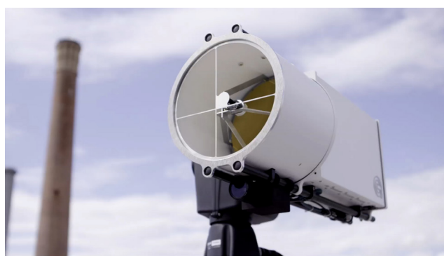
Figure 4. The scanfield sensor unit is a scanning and imaging infrared spectrometer that allows chemical identification and gas cloud mapping over a distance of up to several kilometres.
