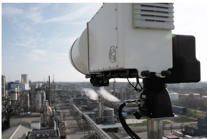
Figure 1. Mounted at an elevated position, the scanfeld sensor unit continuously monitors large areas for dangerous emissions.
