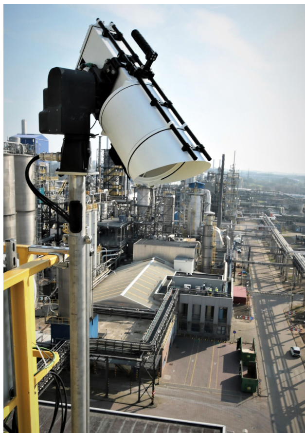
Figure 4. The sensors detect dangerous gases regardless of background – against sky, technical installations, buildings or ground.
