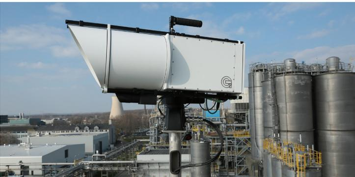
**Figure 2.** Grandperspective's sensors are able to continuously and autonomously identify, monitor and quantify hundreds of gases – including methane, ammonia and ethylene.
