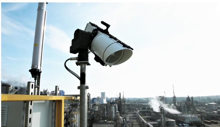
**Figure 5.** Mounted at an elevated position, the scanfeld sensor unit continuously monitors large areas for dangerous emissions.
