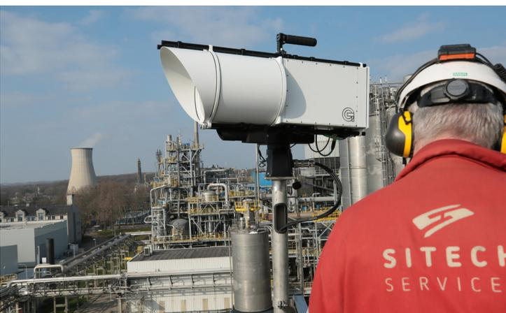
**Figure 3.** A scanfield sensor unit overlooking Chemelot Industrial Park in the Netherlands.
